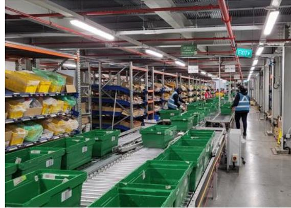
*Pick To Light's (PTL) multi-shuttle system in operation*
